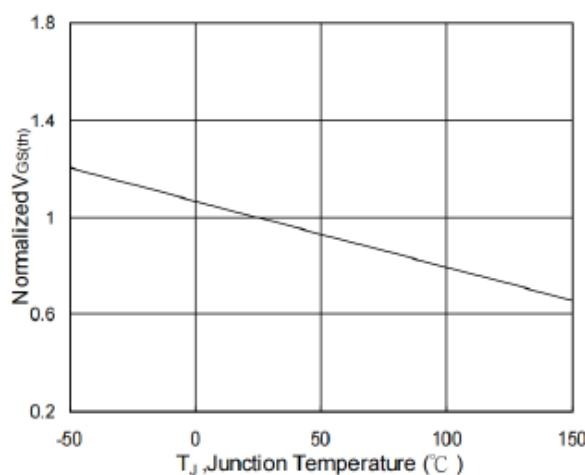
Fig.5 Normalized  $V_{GS(th)}$  vs.  $T_J$
